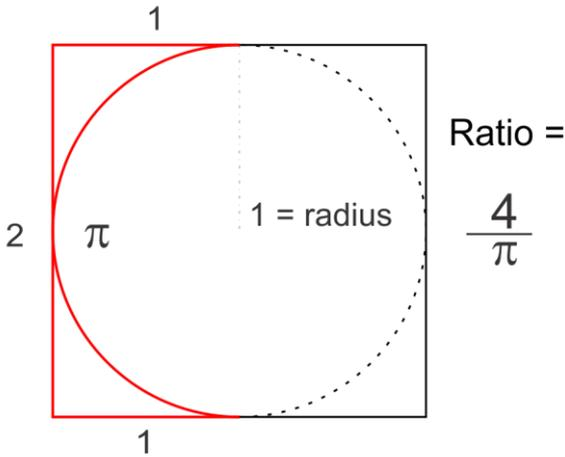
The square signifies the extra cost of travel in rectangular grids. The ratio is the average distance traveled versus the proverbial crow.
