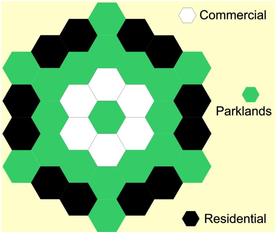
Hexagonal grids allow for 3-way intersections and continuous traffic flow. 3-way intersections have three  $60^\circ$  right turns and three  $60^\circ$  left turns.
